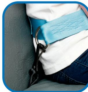
5. With passenger properly seated (hips low against back of seat and shoulders flush to seat) attach the tether hooks to the hip level D-rings.
