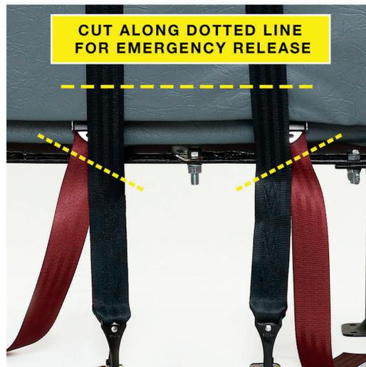
*If passenger is over 168 lbs and is also wearing seatbelt, the vehicle seatbelt will need to be cut as well*
