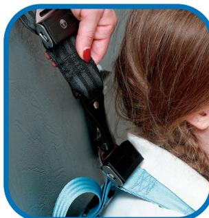
7. From the top of the seat take the 2 tether hooks and fasten them to the tether slots in the shoulder adjusters.
