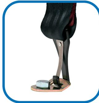
2. Attach (2) tether hooks which have the burgundy and black straps coming from it, to the installed tether hardware kits.
